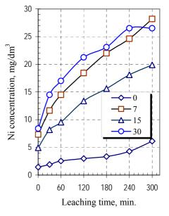
Fig. 10. The effect of Fe(III) on the atmospheric leaching of cobalt from Lubin middlings. (90 °C, s/l = 1:4, oxygen  $-30 \text{ dm}^3/\text{h}$ ,  $H_2SO_4 - 50 \text{ g/dm}^3$ ))
