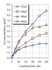
Fig. 4. The effect of temperature on the atmospheric leaching of copper from Lubin middlings. (s/l = 1:4, oxygen  $- 30 \text{ dm}^3/\text{h}$ , H<sub>2</sub>SO<sub>4</sub>  $- 50 \text{ g/dm}^3$ ))
