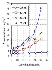
Fig. 5. The effect of temperature on the atmospheric leaching of arsenic from Lubin middlings.  $(s/l = 1:4, oxygen - 30 \text{ dm}^3/\text{h}, H_2SO_4 - 50 \text{ g/dm}^3)$
