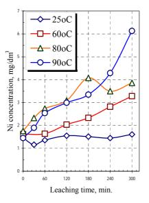
Fig. 7. The effect of temperature on the atmospheric leaching of nickel from Lubin middlings. (s/l = 1:4, oxygen  $- 30 \text{ dm}^3/\text{h}$ ,  $H_2SO_4 - 50 \text{ g/ dm}^3$ ))
