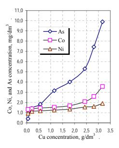
Fig. 12. Corelation between concentration of Cu and other metals during atmospheric leaching of Lubin midddlings at 70 °C, H<sub>2</sub>SO<sub>4</sub> - 50 g/dm<sup>3</sup>
