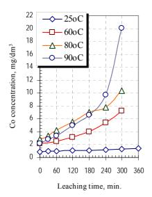
Fig. 6. The effect of temperature on the atmospheric leaching of cobalt from Lubin middlings. (s/l = 1:4, oxygen  $- 30 \text{ dm}^3/\text{h}$ ,  $H_2SO_4 - 50 \text{ g/ dm}^3$ ))
