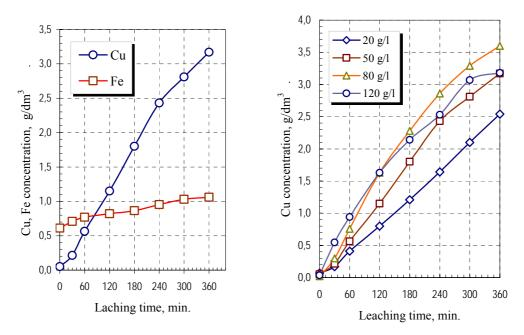
Fig. 2. Cu, Fe concentration – time plots for atmospheric leaching of Lubin middlings in 50 g/l  $H_2SO_4$  solution at 90 °C (s/l = 1:5, oxygen – 30 l/h)
